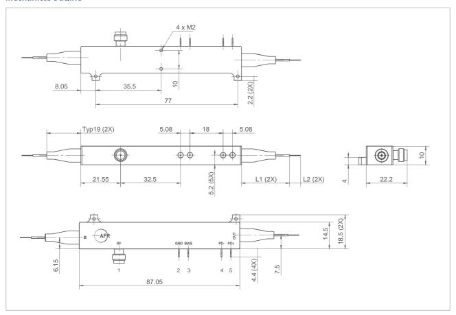
$<sup>\</sup>star$  AM20-XT and AM40-XT have same footprints. All dimensions measured in mm. L1 is fiber length with 900  $\mu$ m loose tube. L2 is length of bare fiber.
